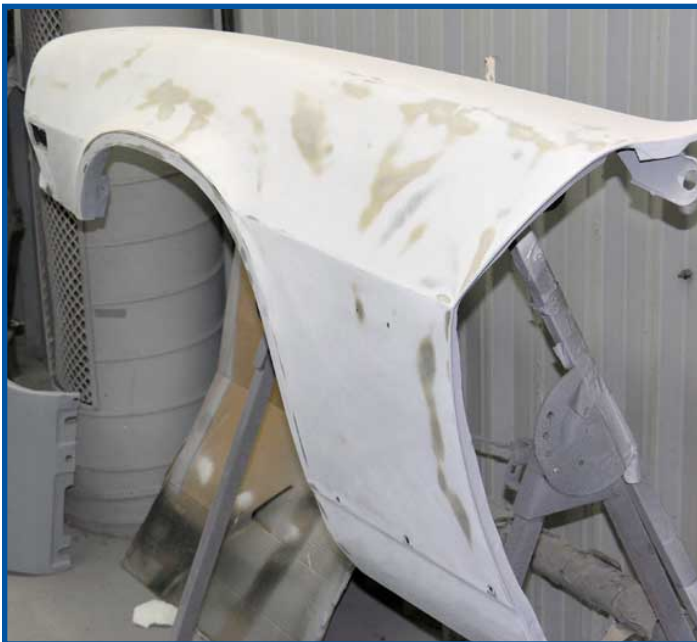
The left fender of Project DZ74 getting prepped for paint.
